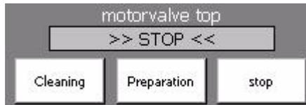
„Cleaning“ The motor valve moves to the Cleaning position
