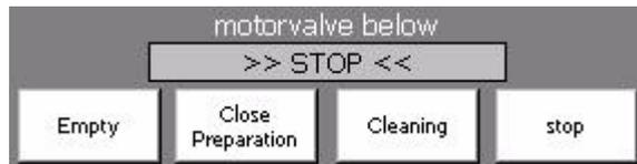
*"Empty"* The motor valve moves to the Empty position
