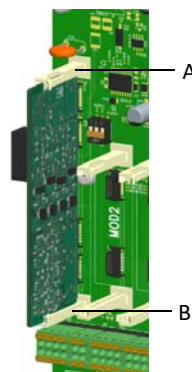
Fig. 10 View, installation of the 4-way mA output card
