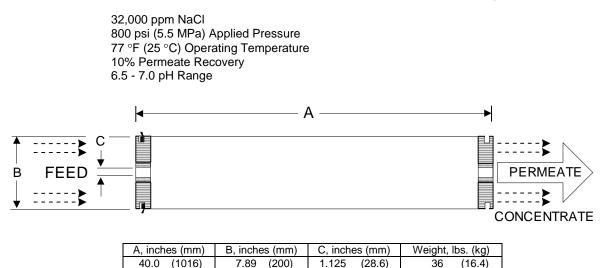
Notice: Permeate flow for individual elements may vary + or - 15 percent. Membrane active area may vary +/-4%. Element weight may vary. All membrane elements are supplied with a brine seal, interconnector, and o-rings. Elements are enclosed in a sealed polyethylene bag containing less than 1.0% sodium meta-bisulfite solution, and then packaged in a cardboard box.
